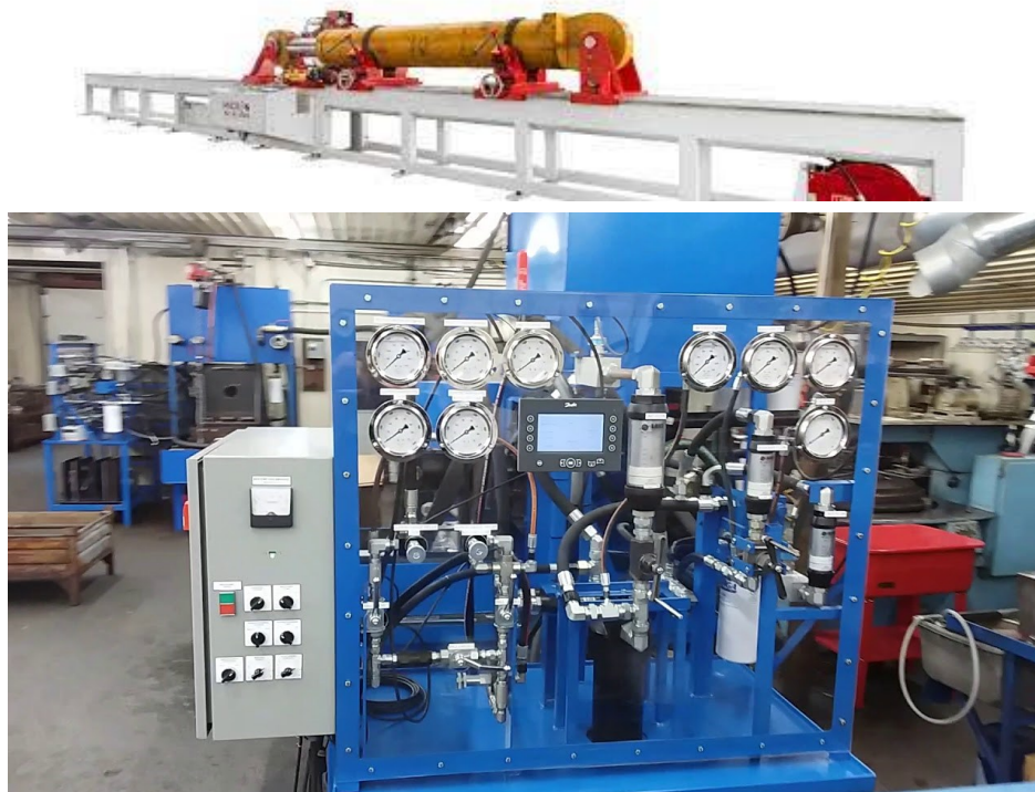
Fig.: Hydraulic Power Unit and Cylinder Stand for the Electro-Hydraulic Cylinder Test Rig
