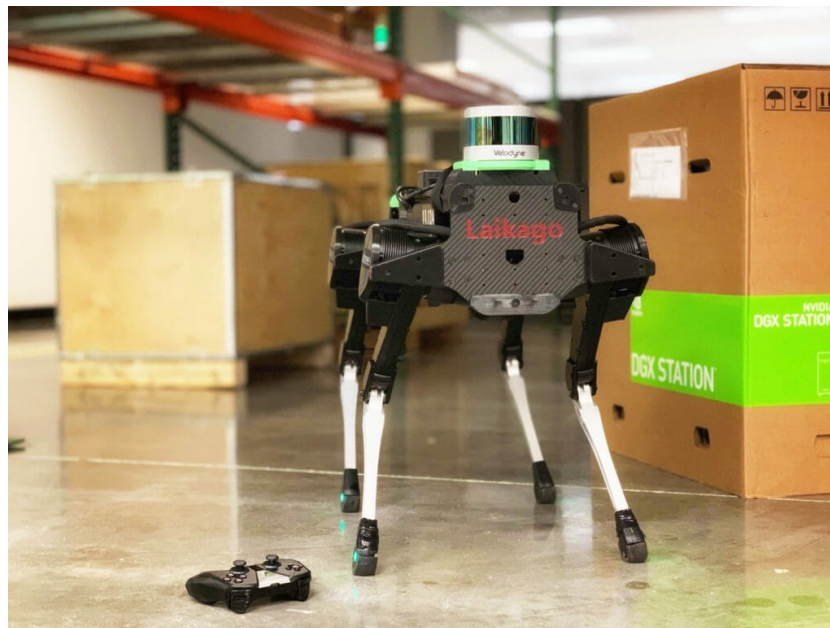
Fig.: Navigation Feedback control for the 4 Legged Robot Locomotor based on the LiDAR Technology
