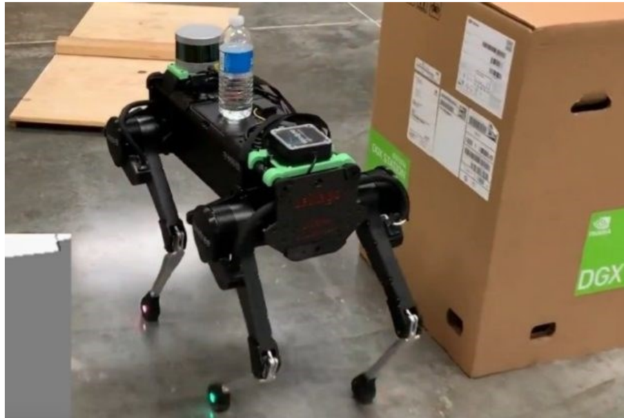
Fig.: Navigation Feedback control for the 4 Legged Robot Locomotor based on the LiDAR Technology
