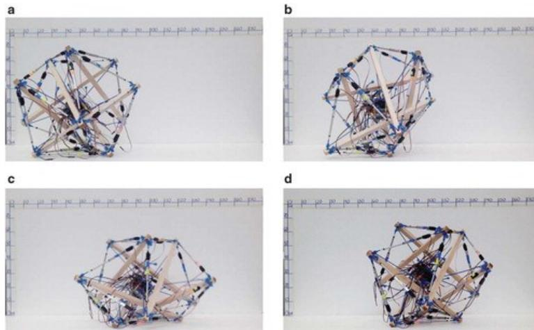
**Fig.:** Spherical Tensegrity Robotics Mechanisms in locomotion
